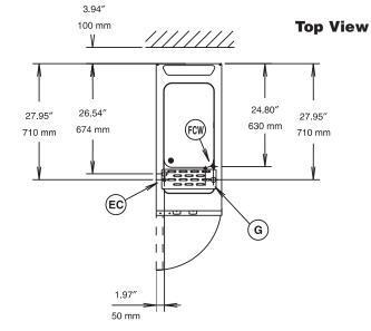
EC = Electrical connectionG = Gas connectionFCW = Filtered Cold Water Inlet
